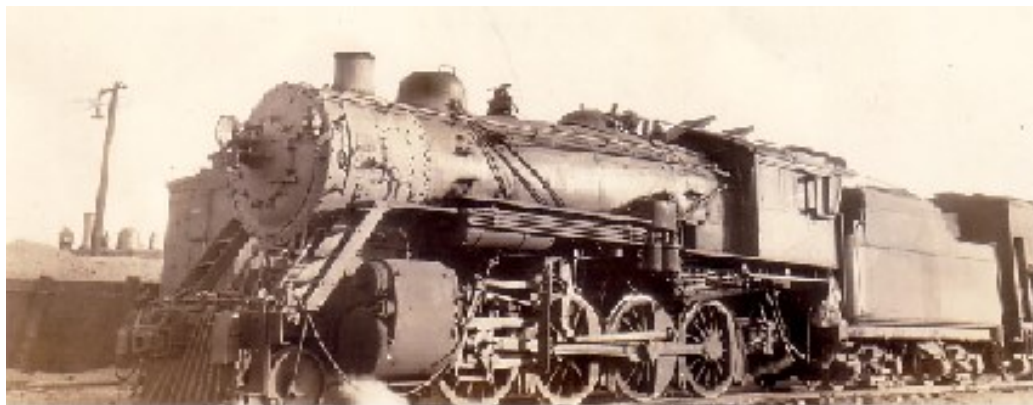
2442 at Shoreham Yard, Minneapolis, MN., 1932. 2442 still has her ORIGINAL, unmodified tender in this photo, along with her Pyle National "Wingboard" headlight. Look closely and you'll see only one smoke box front, signaling that 2442 hasn't had the wreck that resulted in her having two smoke box fronts. Why there is a line connected to the steam dome and running back over the cab and tender the photographer doesn't say, nor why there is an air hose connected to the first air tank and draped over the pilot beam. There is some sort of extra blocking laying on the pilot deck. (from Keith Meacham collection)
