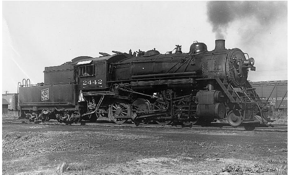
#2442 had a Tractive Power of 43,000 pounds with a length of 67 feet and weighed 351, 263 pounds when loaded with 6,500 gallons of water and 10 tons of coal. This picture of 2442 was taken in North Fond du Lac, WI, 1950 (from Keith Meacham collection)
