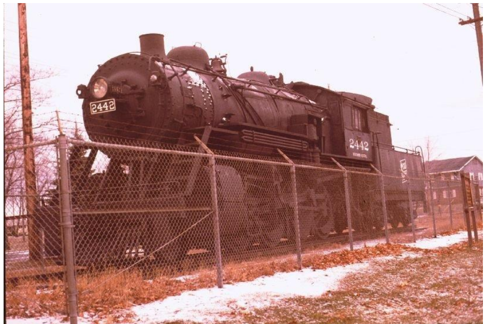
SOO 2442 at Marshfield November 29, 1980—Steam locomotive #2442 is the only example of the Consolidation type 2-8-0— steam locomotive operated by the Soo Line/ Wisconsin Central Railroad. It was built in 1911 by the American Locomotive Company in Schenectady, New York. #2442 was operated from 1911 to 1954. In 1956 #2442 was donated by the Soo Line/Wisconsin Central Railroad to the city of Marshfield and relocated to its present site at Wildwood Park. (from Keith Meacham collection)
